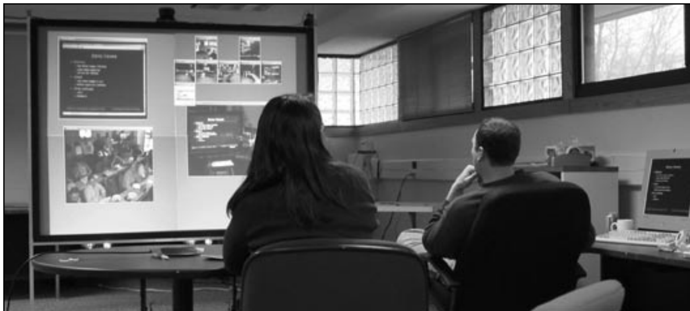
The large tiled display screen in the IRI is used for an Access Grid presentation. The three large windows represent feeds from the host site, including a PowerPoint presentation, a view of the speaker, and a view of the audience at the remote site. The small windows include remote sites that are participating in the session. One of the local cameras is visible at the top of the tiled screen.
